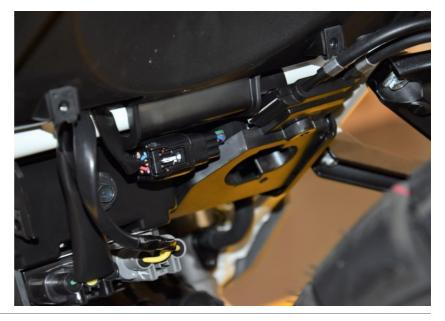
Remove the Exhaust Servo-motor.
