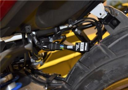
Typical position for the Exhaust Servo Eliminator.
